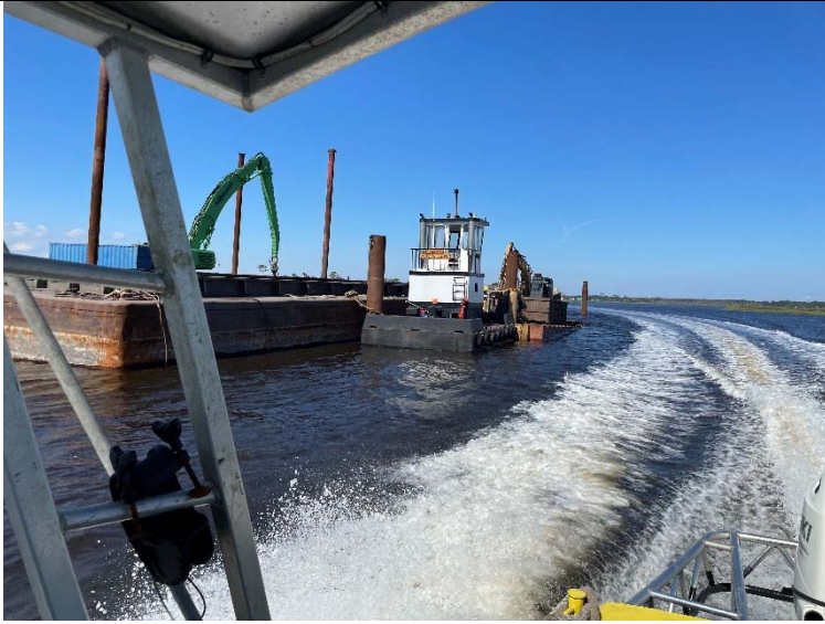
Photo 3: View of 20' Wide Push Barge heading to off-load. Barge currently dredging in Baseline 2: South IOP
